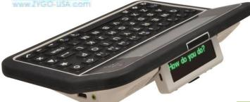
The **Allora 2** is elegantly designed for face-to-face communication! The *detachable display/speaker* can be worn around the neck on a lanyard, or give it to someone to read the message, place it in the middle of the table for a meeting or at the restaurant, or adhere it to the back of the car headrest for the back seat passenger to read. The speech output uses a high quality intelligible **Realspeak** speech synthesizer, and dual forward facing stereo speakers for maximum volume.
